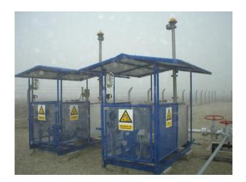
This device has been developed to achieve the simple triethylene glycol usage. It represents an independent type unit with quick mounting ability. The dosing-system has its own steel carrier as well as all the other required attachments on the carrier rim. This enables easy mounting at place where used and it can start operating in a very short period of time.
